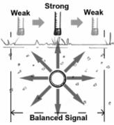
While locating always hold the Receiver vertically, and in the direction of the pipe (in-line with the handle). Swinging the Receiver as you scan may lead you to interpret the signal incorrectly.
