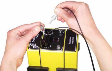
Figure 12-1: Make sure fibre optic strain relief color matches the receptacle door color (grey to grey and black to black).
