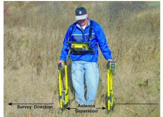
*Figure 11-4: Antennas are held at the proper antenna separation for the selected frequency and perpendicular to the survey line direction.*
