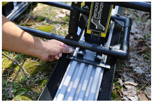
Attach the antennas to the SmartCart <u>before</u> attaching the transmitter and receiver (with batteries inside) to the antennas. To complete all cable connections, see section on <u>Connecting</u> <u>Fibre Optic Cables (</u>3.6.2<u>)</u>. Once completed, the assembled SmartCart is shown below with 50
