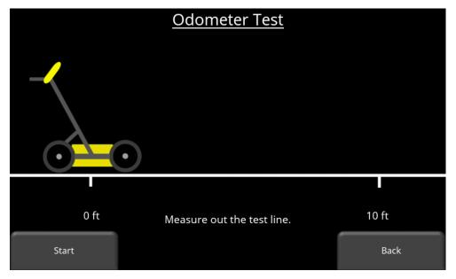
value (Figure 5-24). If the test fails or the percentage difference is larger than the user would like, they should run an odometer calibration (explained below).
