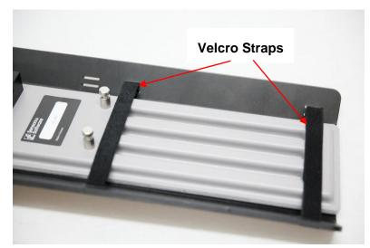
Then attach the antennas to the bottom of the separation bars using the metal posts on the antenna and pins.
