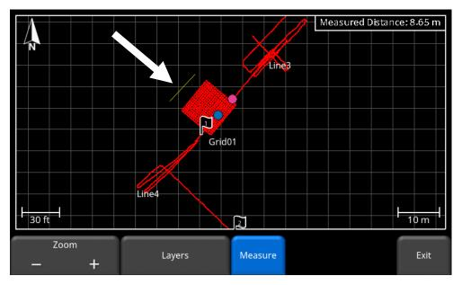
Figure 9-4: The white arrow points to the measure line. The measured distance is shown in the top right corner.
