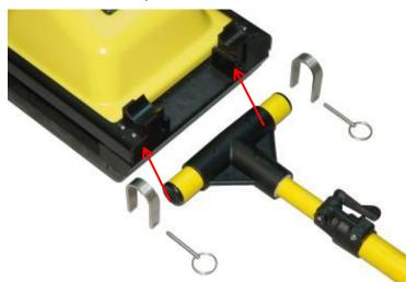
Attach the T-end of the handle to the skid plate assembly by placing the U-bracket over top and into the vertical slots.
