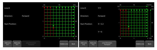
Figure 7-41: Addling lines to a pre-defined grid; before adding lines (left) and after (right)
