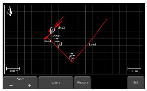
Figure 5-46: MapView showing two grids and multiple lines with interpretations and flags.
