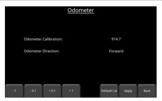
Figure 5-27: Manually setting odometer calibration value
