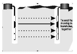
Another example is, if you are scanning a column (Figure 6-14), as you move the transmitter 10cm up the column, the receiver also moves the corresponding distance in the same direction.
