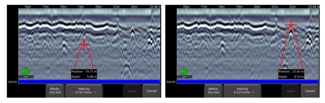
Figure 7-17: Adjusting Velocity, without backing up. Image on left shows initial hyperbola that appears, while the one on the right has the correct hyperbola fit
