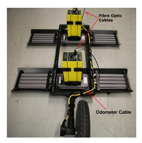
and handle with Velcro straps. The cable should have some slack to reduce any stress during data collection, as the handle assembly moves up and down.
