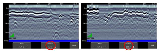
Figure 7-12: Varying the position, or horizontal scaling
