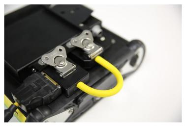
The female end of that cable can connect to the receptacle on the sensor head. When disconnecting the TR1000 cable from the TR1000 or the Adapter Cable, it is necessary to squeeze the connector release tabs on either side of the connector.
