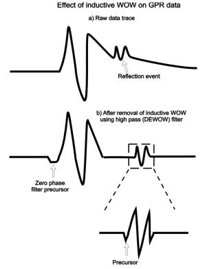
The following image displays a single data trace with the low frequency WOW component present:
