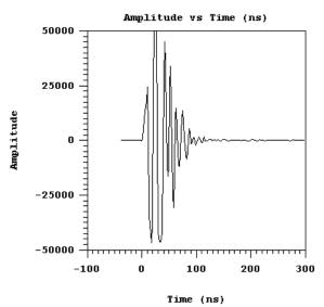
The following image displays a data section where Wow has been removed with the Dewow high pass filter:
