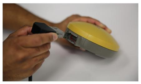
This single cable powers the GPS (if this option is turned on in the GPS menu) and receives data from it. Ensure that the DVL is powered down when connecting or disconnecting the GPS cable.
