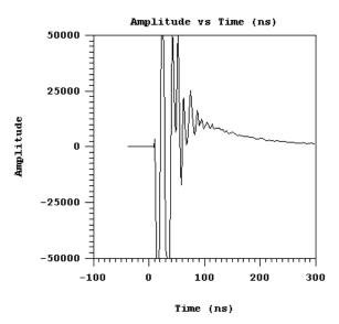
The following image displays a data section with the low frequency WOW component present:
