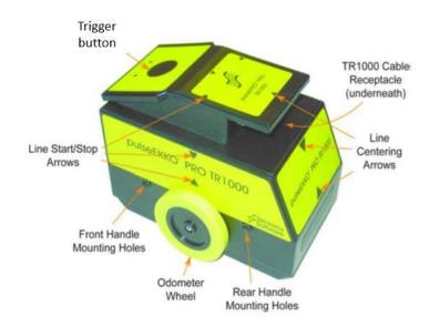
The trigger button on the TR1000 can serve three functions in collection mode:
