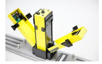
Place one 12-volt battery on each side of each of the electronics boxes. Make sure the positive (+) terminal faces inward toward the electronics.
