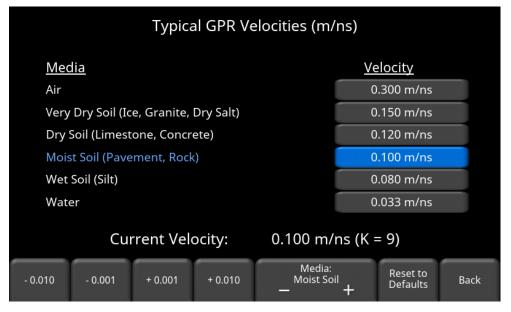
Figure 6-11: Setting GPR velocity (in US Standard units)
