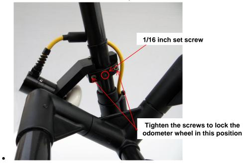
4. Tighten the 1/16 inch set screw into the fibreglass tubing to prevent the odometer from rotating from this position.
