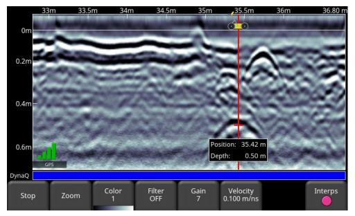
Figure 7-8: Back-up Indicator and Depth Indicator shown
