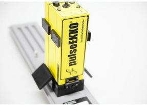
Connect the electronics boxes to the mounting block using the two plastic draw latch connectors.
