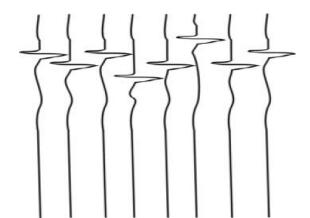
Figure 12-2: Time zero jitter is caused by damaged fibre optic cables.
