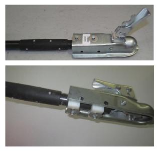
6. Tighten the bolts with a 7/16-inch wrench.
