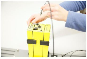
2. Install the fibre optic connection by pushing gently until the connection clicks into place.
