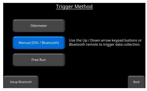
Figure 6-18: Selecting the Manual Trigger
