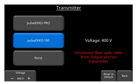
Figure 6-9: Selecting the older pulseEKKO 100 Transmitter.
