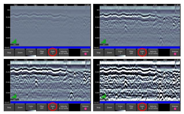
Figure 7-15: Varying the Gain
