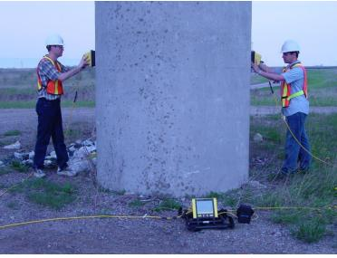
Figure 6-14: Transillumination survey on a column
