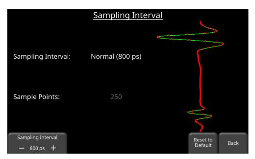
Figure 6-6: Setting the Sampling Interval
