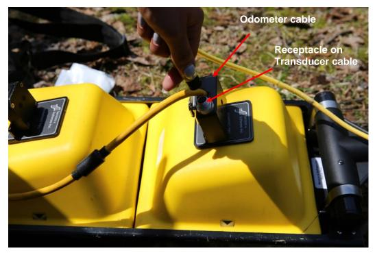
Loop the odometer cable so it does not interfere with the rotation of the odometer wheel. <u>Calibrate the odometer (5.2.2)</u> to ensure accurate data images.
