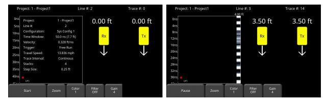
Figure 7-25: Start of Transillumination survey-ZOP (left); after collecting some data, showing antenna positions (right)
