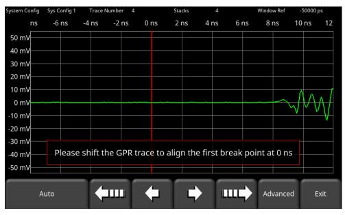
Figure 5-30: Scope mode before First Break correction
