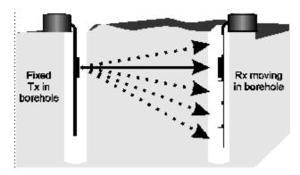
• **Transillumination – VRP** – Short for Vertical Radar Profile. In this survey, the transmitter is fixed and the receiver is moved in steps at right angles to the transmitter orientation. In the case of borehole radar, the transmitter is on the surface and the receiver is moved down the borehole. The transmitter is then moved to another position at a specified interval on the surface and the process is repeated.
