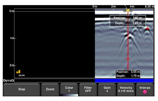
Figure 7-9: Touch the screen for 2 seconds to get depth and horizontal position at any point
