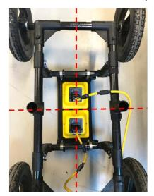
Figure 7-35: Lining up Cart properly on grid lines, shown as red dashed lines.
