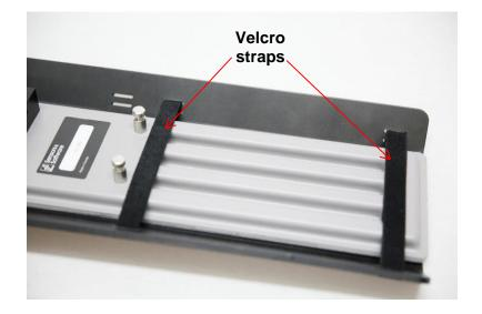
The antennas are secured with Velcro straps to the skid plates. The picture below shows an assembled SmartCart with antenna skid plates.
