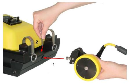
Secure the odometer by inserting the metal pin into the vertical hole on the edge of the skid plate (2).
