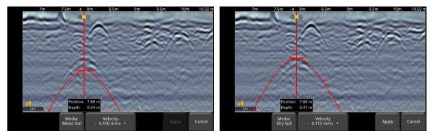
Figure 7-16: Adjusting Velocity while in backup mode. Image on left shows initial hyperbola that appears, while the one on the right has the correct hyperbola fit.
