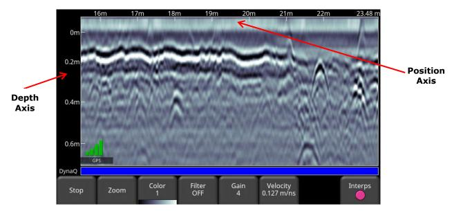
Figure 7-5: Line Scan acquisition mode, showing collected data and axis labels. Touch the vertical scale to switch from depth to time. DynaQ indicator is shown at the bottom above the menu options (odometer trigger only).
