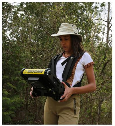
The DVL will connect to a mounting platform, which will then connect to the harness. The viewing angle of the DVL can be adjusted to suit the user.
