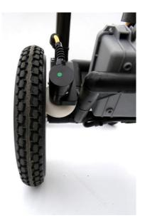
If the odometer contact with the wheel is too loose, the odometer wheel may slip resulting in incorrect position measurements. If the odometer wheel seems loose:
