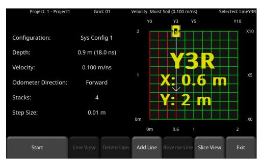
Figure 7-42: Collecting a reverse line around an obstruction
