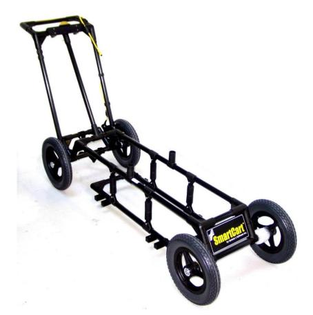
Each system has a unique set of separation bars to attach the transducers or low frequency antennas to the SmartCart and suspend them over the surface.
