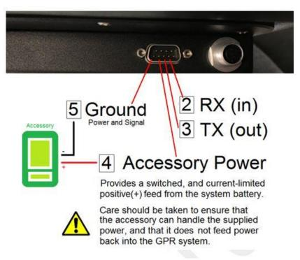
Pressing the **Serial Port Power** button will turn power to the serial port on, but it will display a warning message first (Figure 5-41). Upon restarting, the serial port power will remain at whatever setting the user chose before restarting.
