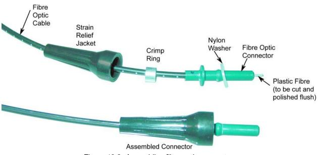
Figure 13-2: Assembling fibre optic connectors
