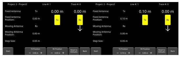
Figure 7-26: Start of Transillumination-MOG (left). After all receiver positions are collected, the transmitter is moved 0.1m (right), and the process repeated.
