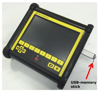
Figure 10-5: Insert a USB memory stick into the USB port on the DVL to export data.
