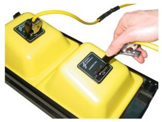
Connect the male end of the transducer cables from the transmitting and receiving transducers to the back of the DVL. The electronics recognize which device is connected to which receptacle. Secure the cable attachments with latches.
