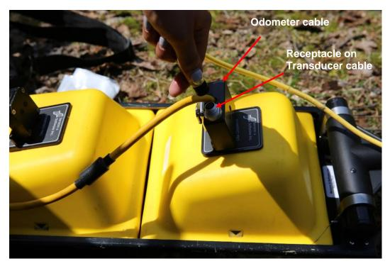
Secure the cables to the cart using Velcro strips or electrical tape. Complete all transducer cable connections as described in the section <u>Connecting Transducer Cables (3.6.3)</u>.
