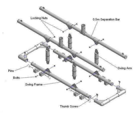
1. Make sure the Swing Arm bold head is caught by the plastic ridge, so it cannot rotate. Do not over-tighten, the Swing Arm needs to move freely.
