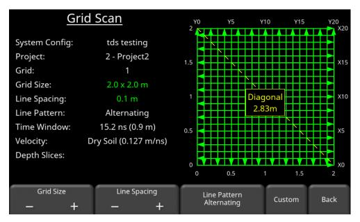
Figure 7-30: Forward/Reverse grid line collection
