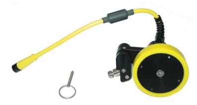
Attach the small wheel odometer to the skid plate assembly by inserting the metal post into the hole on the end of the skid plate (1).
