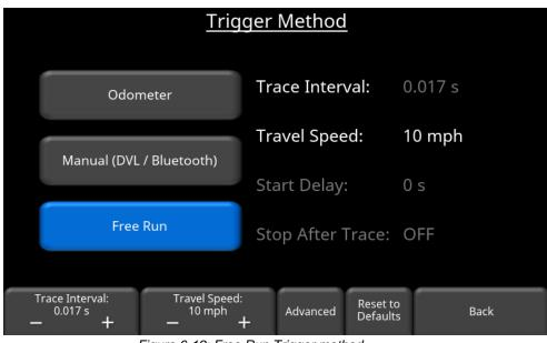
Figure 6-19: Free Run Trigger method
