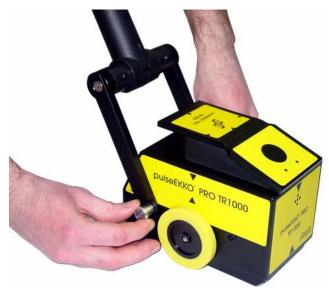
There is an additional set of handle mounting holes at the front of the TR1000 which can be used when scanning a vertical surface or in confined spaces when it is preferable to pull the TR1000 towards the user rather than pushing it.
