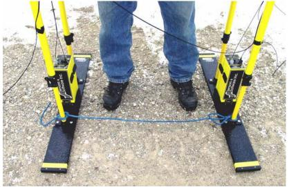
Figure 11-2: Using string to keep antennas at fixed separation
