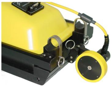
Loop the odometer cable so it does not interfere with the rotation of the odometer wheel. Connect the odometer cable to the receptacle on the transducer cable. You can also connect the odometer cable to the back of the DVL, but you will need an odometer extension cable; this is not recommended as the cables now need to run a longer distance, near the antennas.
