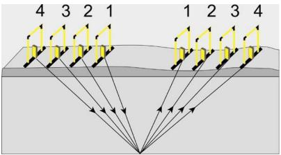
Figure 11-5: Illustration of a CMP Survey
