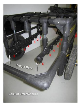
Attach the hangers to the hanger bar using the nuts and bolts provided. Use two 10 mm wrenches to assemble the hangers (wrenches not provided).
