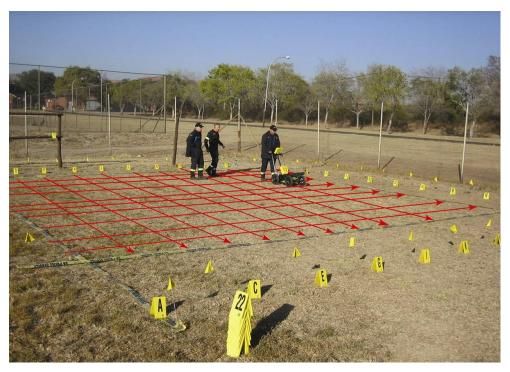
Figure 7-34: Example of a grid survey. The red lines are superimposed just to illustrate the concept.
