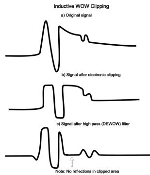
The original signal acquired by the antenna and then sent to the receiver electronics is similar to diagram **a**) above.
