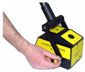
An assembled TR1000 with handle is shown below. When using the handle, a harness is typically used to support the DVL in front of the operator <u>Section</u> 3.7.2.
