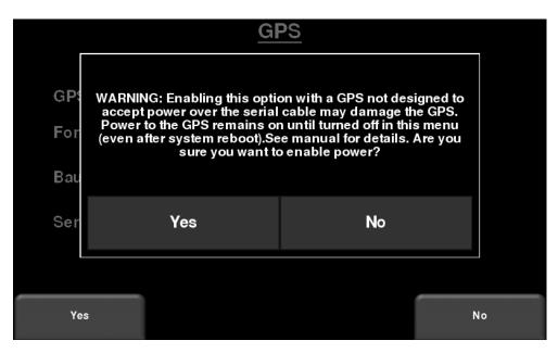
Figure 5-41: Warning message if you enable power to the serial port
