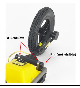
Face the labels on the transmitting transducer toward the odometer wheel. Secure the cable to the T-bar with Velcro straps.
