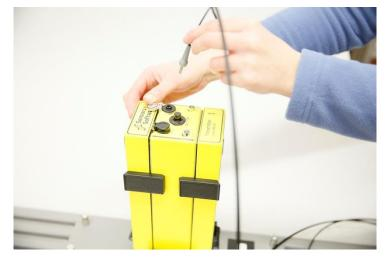
You can use an older pulseEKKO 100 transmitter with the pulseEKKO PRO and Ultra Receivers (see <u>Transmitters</u>,6.1.6).
