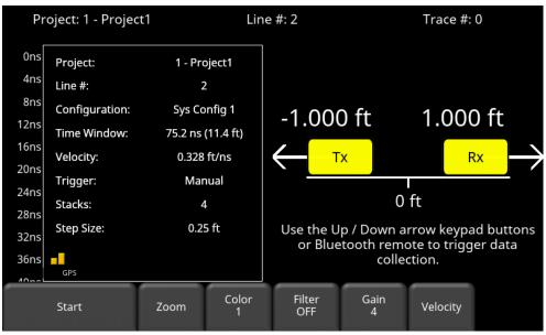
Figure 7-23: Collecting line data in a CMP survey
