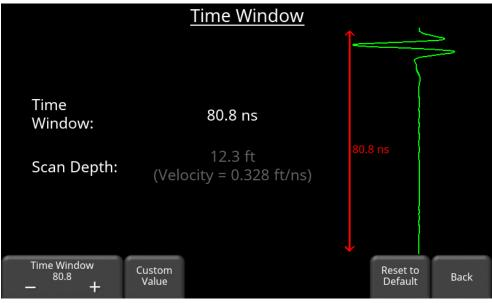
Press Time Window to display the screen in Figure 6-3, where you can set the Time Window in nanoseconds.
