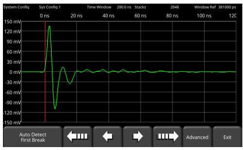
Figure 5-31: First Break at the correct position
