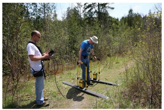
Figure 11-1: Two-person data collection with the pulseEKKO system. The antenna operator moves the antennas one Step Size to each new data collection position.
