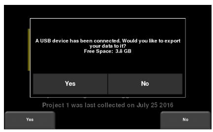
Figure 10-6: When a USB drive is connected to the DVL, a message opens asking if you would like to export all your data to it.
