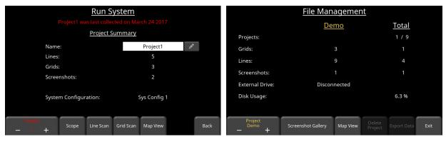
Figure 9-1: Accessing Map View either from the Run System screen (left) or File Management menu (right)
