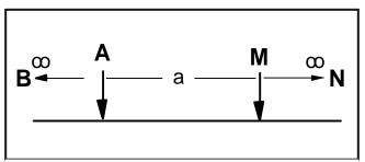
Figure 13 Pole-pole electrode array
