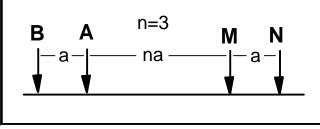
Figure 11 Dipole-dipole electrode array
