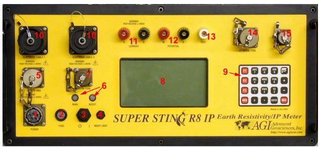
Figure 8 SuperSting R8/IP front panel
