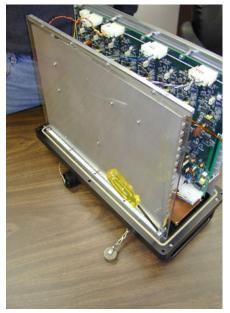
Figure 46 Unscrew the five hex screws, holding the transmitter board mounting plate to the front panel.
