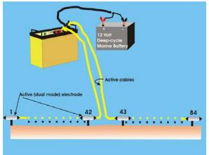
Figure 3 SuperSting set-up with active (dual mode) electrodes
