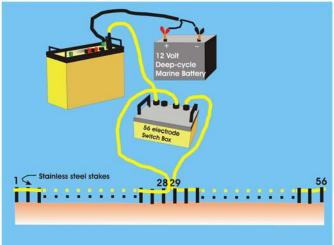
Figure 27 SuperSting/Switch box connection
