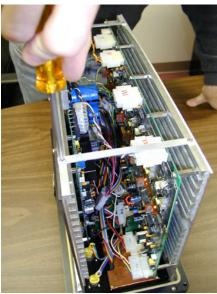
Figure 45 Unscrew two screws holding the bars to the transmitter board on the left side.
