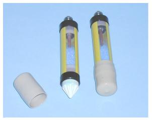
Figure 44 Non-polarisable electrodes
