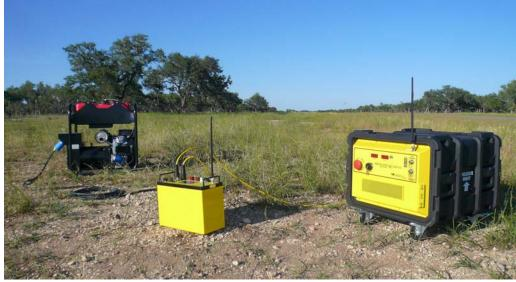
Figure 21 The SGS generator, SuperSting R8 and a PowerSting makes up the system.
