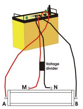
Figure 35 Connect SuperSting to the soil box using the voltage divider for the M and N terminal.
