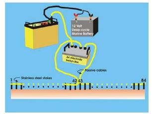
Figure 4 SuperSting set-up with external switch box and passive cables
