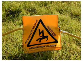
Figure 1 Use the electrode warning covers
