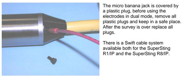
Figure 40 Remove the plastic plug using your finger nails
