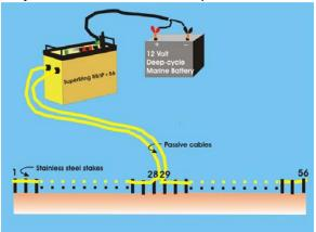
Figure 5 SuperSting set-up with built-in switch box and passive cables
