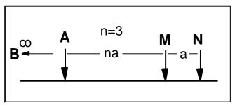
Figure 12 Pole-dipole electrode array
