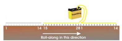
Figure 6 Data is first collected using cable section 1-14 and 15-28 to the left in the picture. After the initial data is recorded cable section 1-14 is moved to the right and connected to the SuperSting which also has been moved forward
