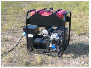
Figure 25 The Sting Generator Set is a compact power unit.
