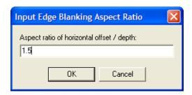
This control also prompts for a blanking aspect ratio of horizontal offset to depth. Set the ratio to 1.0 for a 45° blanking, which may not appear as 45° due to the vertical exaggeration. A blanking aspect ratio larger than 1.0 seems more appropriate. Choose a larger ratio to hide inversion artifacts.
