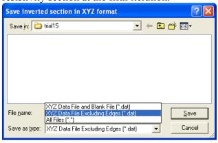
The tool button ( $^{\mathbf{m}}$   $^{\mathbf{f}}$ t) on the graphics toolbar changes the length unit from meters to feet or from feet to meters. The saved data in XYZ format will have the length unit of the user's choice.
