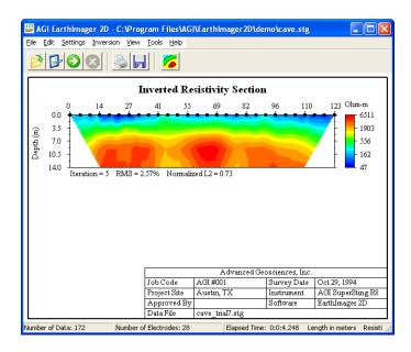
This turns on or off an edge blanking feature for surface data. So the resulting section looks similar to the apparent resistivity pseudosection. Surface surveys do not have good resolution at two ends of the survey line, so inversion artifacts are often seen at two ends. It is preferred not to show these artifacts as they mislead the data interpreter.
