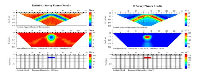
8) For IP survey planning, inverted resistivity and chargeability sections are shown at the end of IP inverse simulation.
