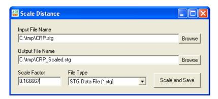
Choose the data file you want to scale its electrode coordinates as the input file. A default output file name will be recommended. Then choose a correct scale factor. Make sure the file type is right. Currently EarthImager support both STG data file and CRP water depth file. Finally click Scale and Save button, the electrode coordinates will be scaled to correct distance and a scaled data file will be saved in your designated folder and file name.
