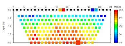
Scatter Plot of Surface Apparent Resistivity Data
