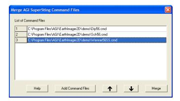
To merge several SuperSting command files, simply add command files to be merged to the List of Command Files by clicking the Add Command Files button. The up and down arrow buttons may be used to move a command file up or down on the list. The order of command files will determine the data collection sequence during the actual survey in the field. Finally, click the Merge button to save a mixed array command file.
