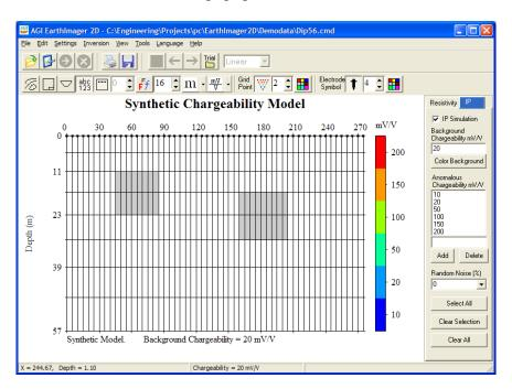
21) Choose Forward Simulation from the Tool menu. This will start the forward simulation. For surface surveys, you will see an apparent resistivity pseudosection at the top and the actual model on the bottom of the main window. If the IP simulation is activated, resistivity forward simulation is carried out first, then IP forward
