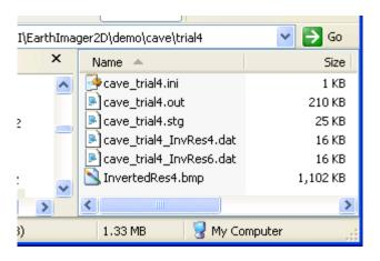
The INI file is the inversion settings file and may be read back into the EarthImager for inversion of other data sets. The OUT file is an inversion log file containing inversion settings, raw data, mesh definition, inverted results of all iterations. The STG file contains the actual data used in
