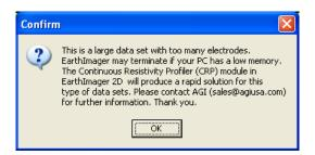
If your data set consists of too many electrodes and your dongle was activated for CRP, EarthImager will automatically enter the CRP processing mode. There is a CRP check box on the Settings | Initial Settings window for deactivating the CRP mode. If this CRP check box is unchecked and you read in a large data file with many electrodes (say, over 200), a dialog box would pop up to ask you to confirm:
