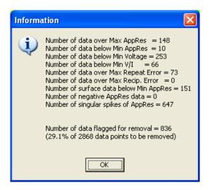
The number of data flagged for removal is counted based on the Criteria for Data Removal in the Initial Settings Window. Any edits from the Electrode Editor or manual editing will be added to this number. But any change in the Criteria for Data Removal will reset this number.
