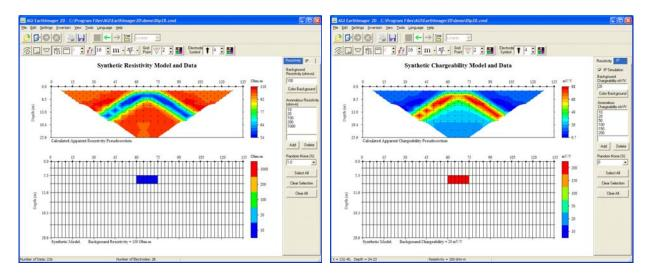
22) For borehole resistivity imaging, the synthetic model will be shown to the left and the apparent resistivity or chargeability scatter plot to the right.
