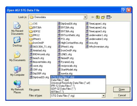
To read a non-STG data file, go to File | Read Data menu or click the Read-Data tool button Then choose "Universal Resistivity Files" from the "Files of Type" box (see below). You may find other resistivity data file formats supported in EarthImager 2D.
