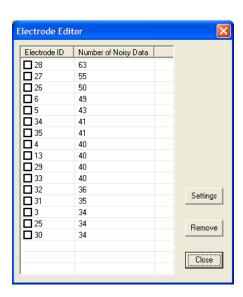
The third utility to identify and remove the noisy data is a manual data editor using mouse clicks and the Delete key. You can edit the raw data before the inversion, and remove poorly fit data on the data misfit scatter plot after the inversion and start the inversion again with the "clean" data.
