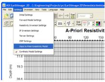
A borehole data set cannot be displayed in a pseudosection, so it almost always starts from a homogeneous half space of the average apparent resistivity value.
