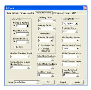
One of the objectives of the resistivity inversion is to find a resistivity model whose response (predicted data) best fits the measured data. The goodness of the fit may be characterized by the **root mean squared** (RMS) error in percent (%) defined below.
