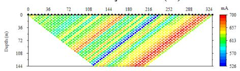
The measured voltage scatter plot below shows a strange low-voltage feature in the middle of the pseudosection. This is caused by unqualified and asymmetric infinity electrodes which are not placed far enough from the survey area. The scatter plot of geometric factor below shows a zone of high geometric factors that result in a low voltage zone.
