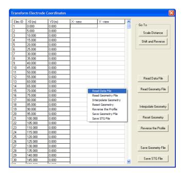
To start the "Transform Electrode Coordinates" utility, choose the menu item Tools | Transform Electrode Coordinates. There are two links on the window for scaling all coordinates with a constant factor (go to Scale Distance) and for Shifting and Reversing a profile (go to Shift and Reverse). You may also find these two tools under the Edit menu.
