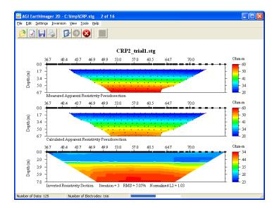
For each subsection, EarthImager saves these six files: an inversion settings file (\*.ini), a clean STG file after removal of some noisy data, an inversion output file (\*.out), a JPG file of inverted resistivity section at the iteration with the smallest RMS error, a data file (\*.dat) of inverted resistivities in the XYZ format, and a blanking file (\*.bln) for compatibility with the Surfer graphics package. The OUT file may be loaded back into EarthImager for further study.
