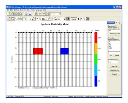
5) If borehole electrodes are detected, the Survey Planner would enter the Electrical Resistivity Tomography (ERT) mode automatically. A typical ERT mesh may look like this.
