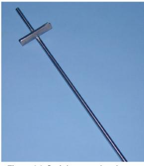
Figure 24 Stainless steel stake, 457 mm x 9.5 mm
