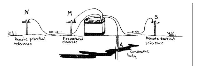
Figure 30 Sting used for mise-a-la-masse measurement. Note that N and B are reference electrodes placed at "infinity".
