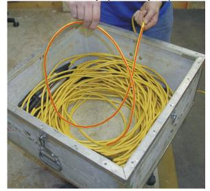
Figure 5 Incoming cable "under" the loop.
