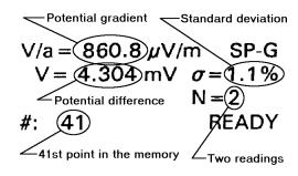
Figure 3 Result display for the SP-gradient array type.
