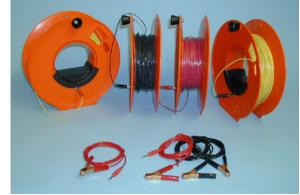
Figure 20 Short cable set, current 2x150 m, potential 2x50m.
