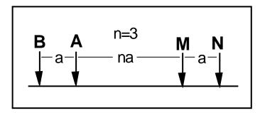
Figure 10 Dipole-dipole configuration
