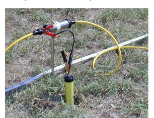
Figure 15 Electrode used in dual mode configuration.
