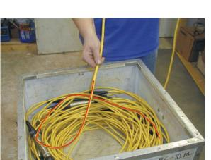
Figure 4 Incoming cable "over" the loop.
