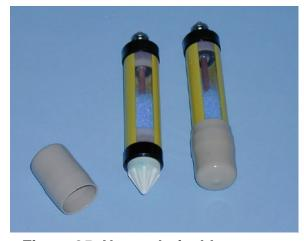
Figure 25 Non-polarisable electrodes.
