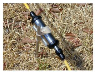
Figure 6 Rubber band each switch to its electrode stake.
