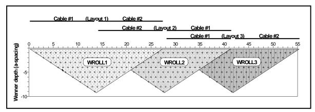
Figure 8 Data coverage using Wenner roll-along with 28 electrodes divided on two cables. Note that the overlapping readings are not measured as they are redundant.
