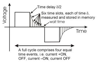
Figure 1 Resistivity/IP measurement sequence.
