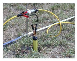
Figure 12 Electrode in dual mode configuration.
