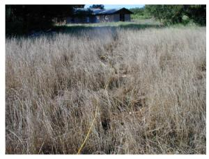
Figure 23 It is not easy to find the stakes once the cable is gone (left picture). Instead follow the cable and pick up the stakes before picking up the cable (right picture).
