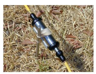
Figure 16 Electrode used in single mode configuration.
