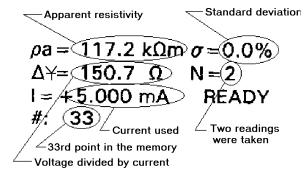
Figure 2 Result display for Schlumberger, Wenner, dipoledipole, pole-dipole and azimuthal.
