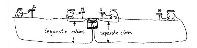
Figure 29 Make sure to separate the cables in order to avoid cross-talk between cables.
