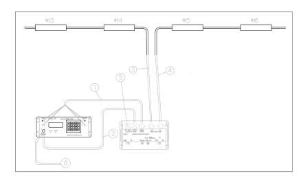
Figure 7 Sting/Swift connection: 1=ABMN cable, 2=Sting/Swift communication cable, 3=Swift cable with low numbers, 4=Swift cable with high numbers, 5=receptacle for PC connection, 6=connector for external 12 V DC battery.
