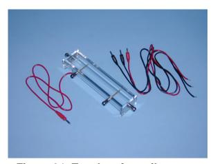
Figure 31 Test box for soil samples.
