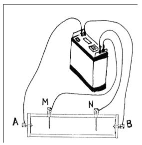
Figure 32 Sting connection to the soil box.
