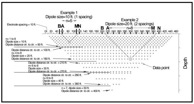
Figure 11 Data configuration for a complete dipole-dipole data set automatically recorded using 47 smart electrodes. Note that the measurement process occurs form left to right, layer by layer form the top; not from top at an angle towards the bottom as is the case in most manual arrays.
