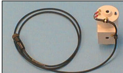
Figure 11. Top sensor with gradiometer cable attached.
