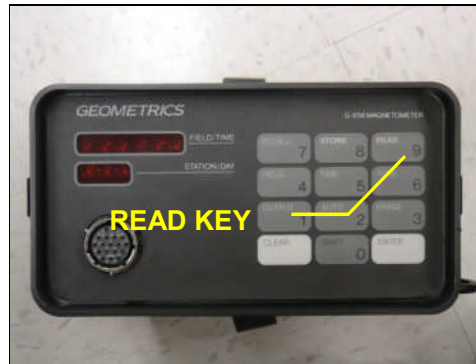
Figure 8. Location of 'Read' key on magnetometer console.
