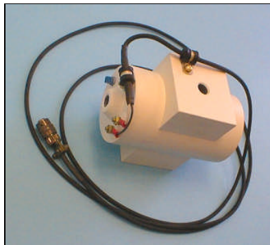
Figure 12. Bottom sensor with gradiometer cable attached.
