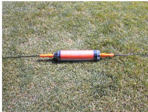
Dipole cables attached to receiver
