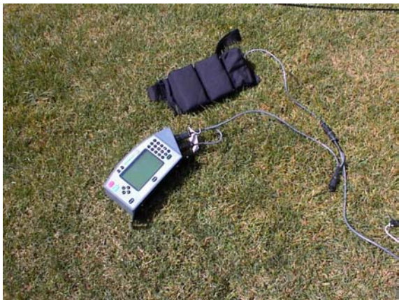
Attach battery cable to console cable
