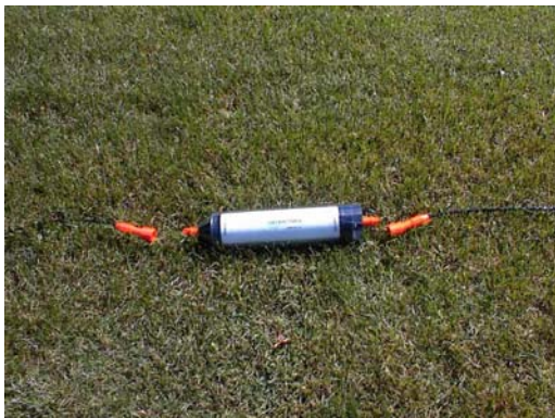
Dipole cables to be attached to transmitter
