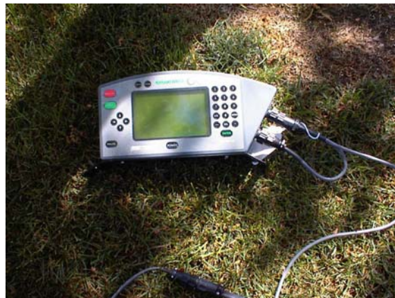
Power and data connections of console cable
