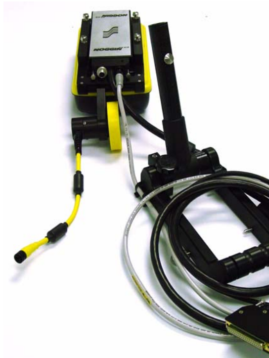
Figure: 2-4 Connect the 37 pin connector on the Noggin-to-DVL cable to the 37 socket receptacle on the Noggin unit by tightening the latch.
