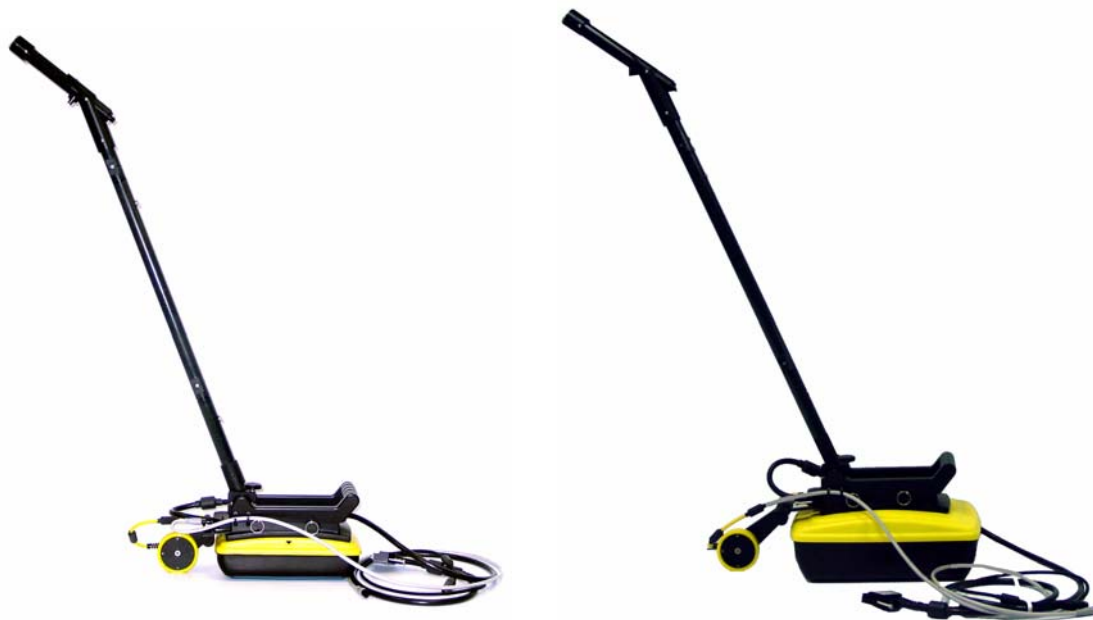
Figure: 2-9 Connect the SmartHandle grip to the SmartHandle extension. The Noggin 1000 is shown on the left and the Noggin 500 is shown on the right. The grip should click securely into place. To release the grip, push the large grey button and pull the two pieces apart.
