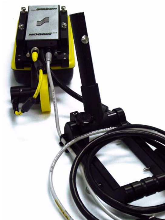
Figure: 2-5 On the Noggin-to-DVL cable, note the round receptacle on the back of the connector that attaches to the Noggin unit. Connect the yellow odometer cable to this round receptacle.
