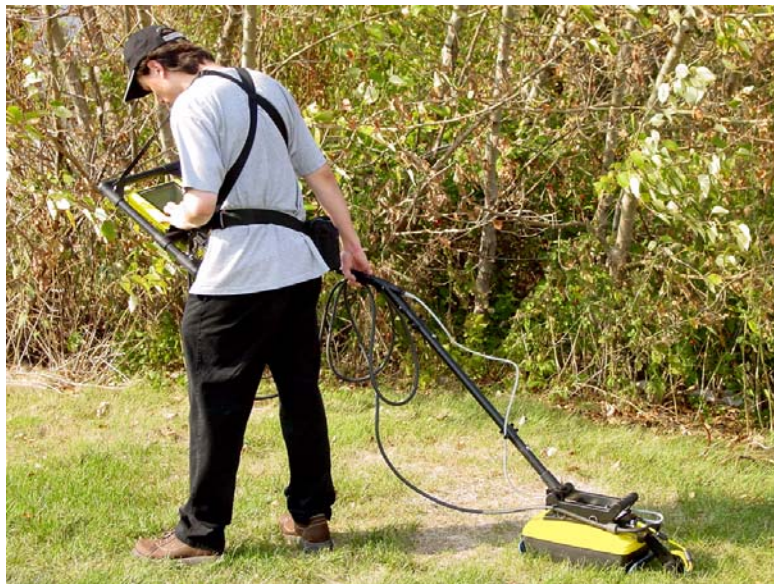
Figure: 2-11 In conditions where pushing the SmartHandle is difficult, it is possible to turn the handle around and pull the system as shown.
