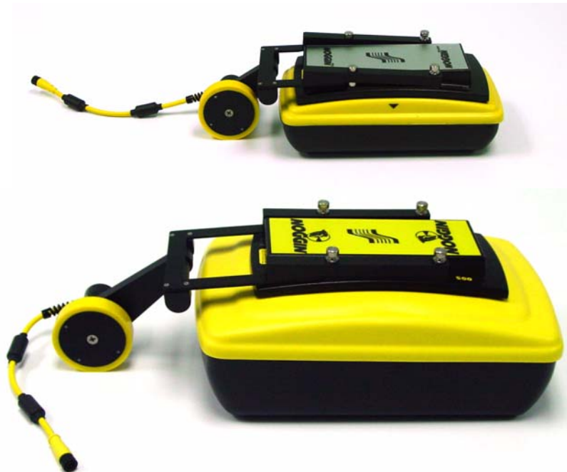
Figure: 2-3 Slide the Noggin odometer bracket over the four, silver mounting posts for both the Noggin 1000 (top) and Noggin 500 (bottom). The odometer wheel should be pointing towards the floor.
