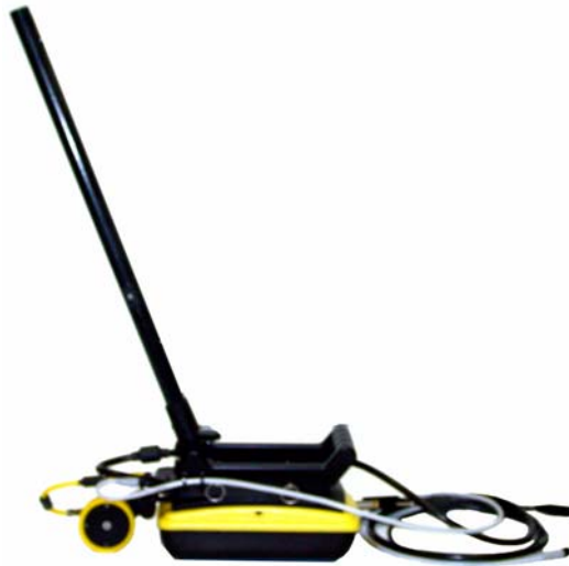
Figure: 2-8 Push the SmartHandle extension into the handle base. The extension should click securely into place. To release the extension, push on the large grey button and pull the two pieces apart.
