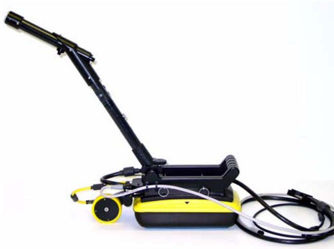
Figure: 2-10 For a shorter handle, just connect the SmartHandle grip to the handle base without the extension.
