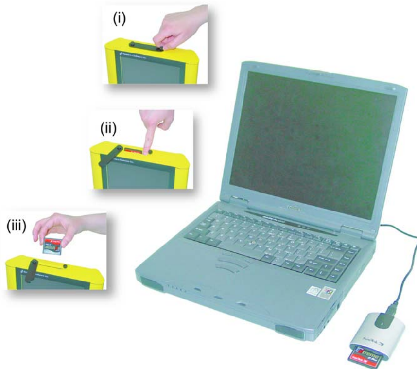
Figure: 5-16 Noggin data files saved to the removable drive are easily transferred to a PC. First, power down the DVL, then (i) loosen both of the finger-screws on the top of the DVL so the drive door can swing open freely. (ii) Press the button to partially eject the compact flash drive. (iii) Remove the drive and insert it into a PC card reader (user supplied). Copy the Noggin data files from the drive into a folder on the PC using the Windows Explorer program. The Win-PXFER program can then be used to view the Noggin data.
