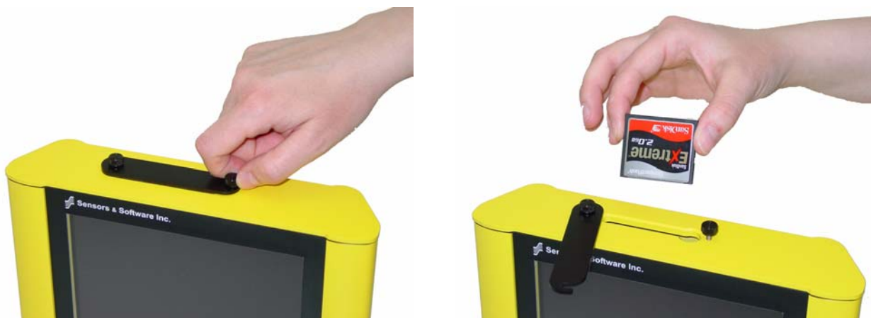
Figure: 3-2 The DVL has a removable compact flash drive for data storage.
