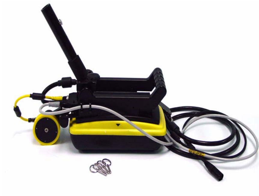
Figure: 2-6 Press the handle base straight down onto the four, silver mounting posts. The handle base should be pushed all the way down onto the odometer bracket.
