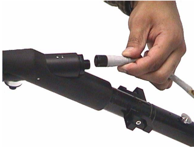
Figure: 2-13 The Smart Grip Cable attaches to the end of the SmartHandle Grip. This connects the Smart button (extreme left, bottom) and beeper (not shown) into the system.
