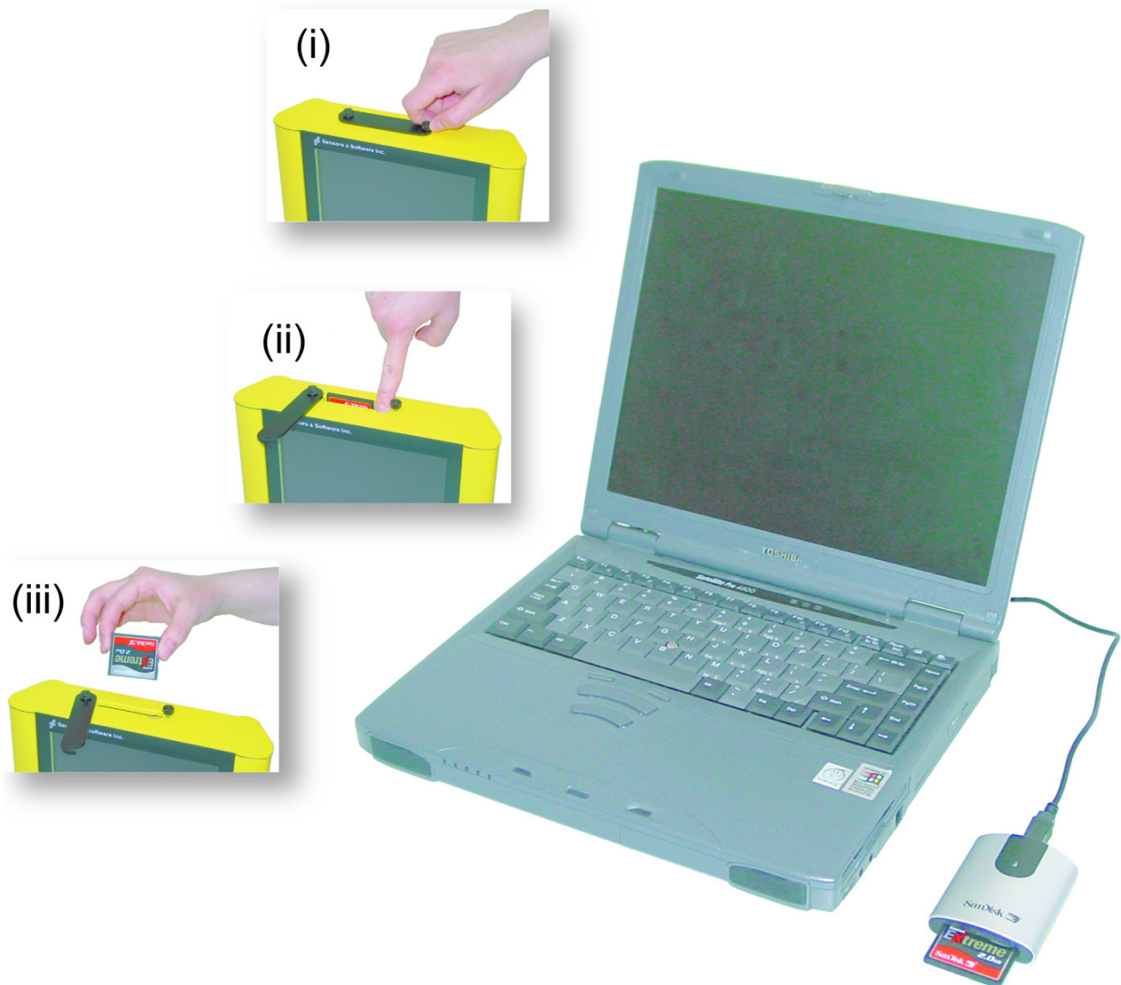
Figure: 4-15 Noggin data files saved to the removable drive are easily transferred to a PC. First, power down the DVL, then (i) loosen both of the finger-screws on the top of the DVL so the drive door can swing open freely. (ii) Press the button to partially eject the compact flash drive. (iii) Remove the drive and insert it into a PC card reader (user supplied). Copy the Noggin data files from the drive into a folder on the PC using the Windows Explorer program. The Win-PXFER program can then be used to view the Noggin data.
