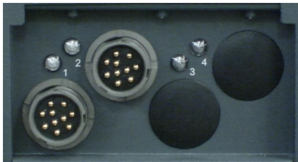
Figure B-13: Digital data connectors.
