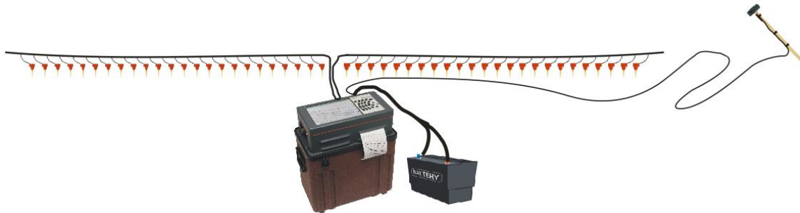
Figure B-16: Typical 48-channel StrataVisor layout.
