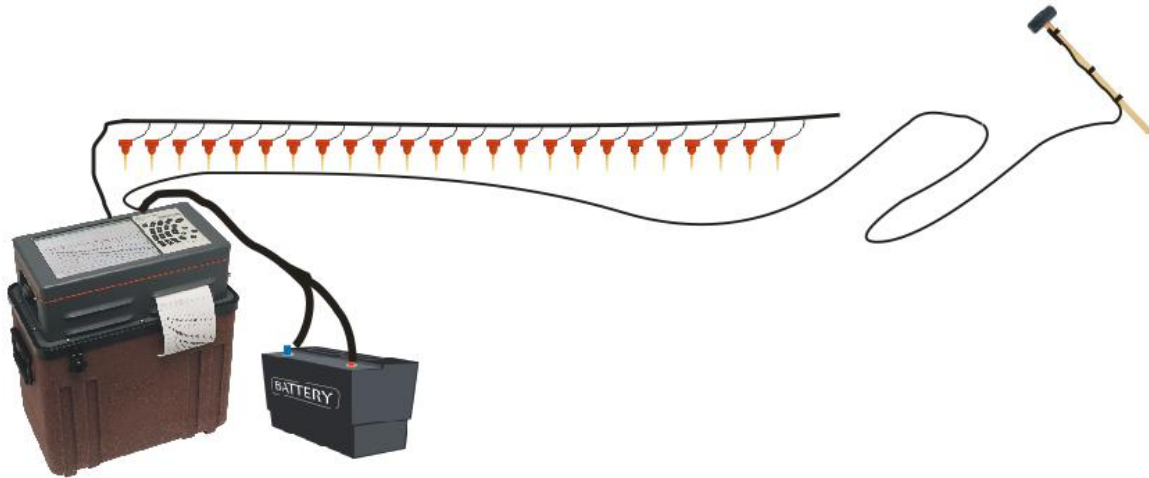
Figure B-15: Typical 8-24 channel StrataVisor layout.
