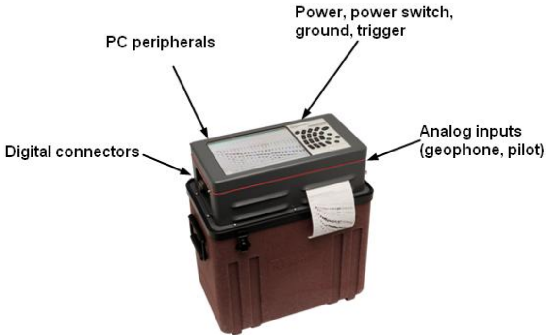
Figure B-9: Annotated photograph of StrataVisor NZ.
