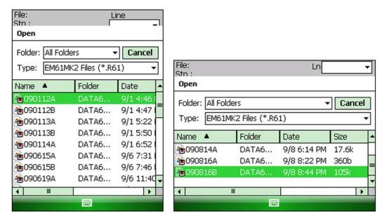
The file name can be selected in the Open Data File dialog using the Windows standard interface procedure. After the file is selected (highlighted) tap the button **OK** or press **ENTER** key to accept and display data file (to cancel selection tap **Cancel** (X) button or press **Esc** key). After the file is opened readings taken at the beginning of the first survey line in the file are displayed, as shown below.
