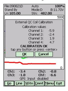
Otherwise, if the program determines that the reading is outside of the test values range the corresponding message "CALIBRATION FAILED" is displayed.
