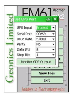
Similarly, the BC-337 GPS (CF card based) occupies the first available serial port as well. The Baud Rate for this device is usually 4800 KBytes. The typical GPS Port Setup dialog configuration is shown below.
