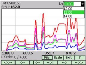
drop-down box showing the available survey lines. When the keyboard is being used you can activate the text box by pressing the **TAB** key until the drop down box is highlighted and then by using Up or Down arrow keys select one of available lines (as shown above).
