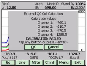
Regardless of the test result (OK or FAILED) the readings will be saved on screen. The program returns to Monitoring window after any button is tapped or ENTER key is pressed. Then the Internal QC coil calibration process can be repeated.
