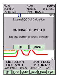
The logger will determine if the instrument has passed test. If after activating the QC coil, the program determines that the reading is inside the standard values within +/- 10% tolerances then a message "CALIBRATION OK" will be displayed.
