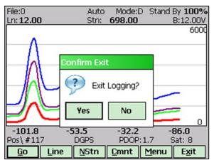
After above message is confirmed the program stops logging, closes data file and returns to Main Screen.
